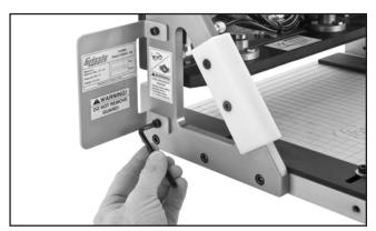
Figure 4. Attaching guard to jig.
